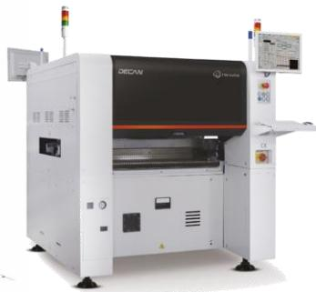
**The Standard Of Flexibility** demonstrations featuring Hanwha's model XM520 pick-and-place system showing the advantages of single and dual lane efficiency, with greater flexibility, extended component range, multifunctional/odd-form capability, mixed production-readiness and compatibility with HM, Decan and SM series platforms.
