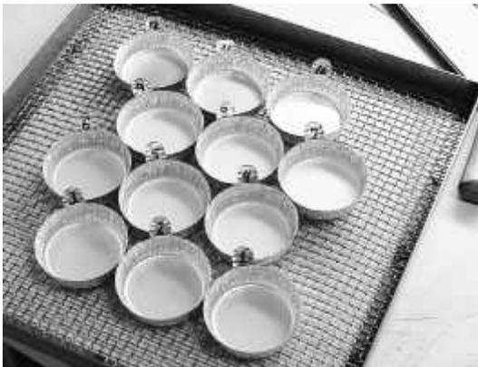
**Samples prepared for NVR testing**
